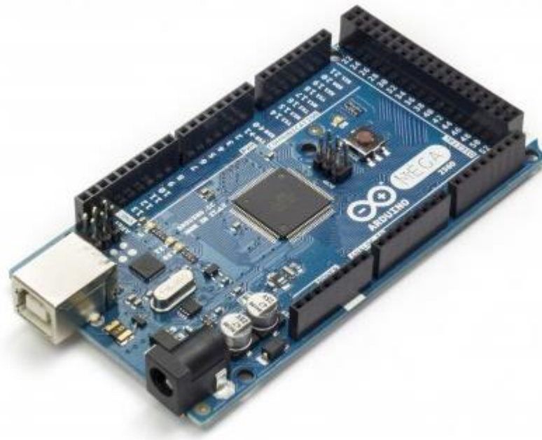
Figure-27: Arduino mega 2560 host board of EKG shield
