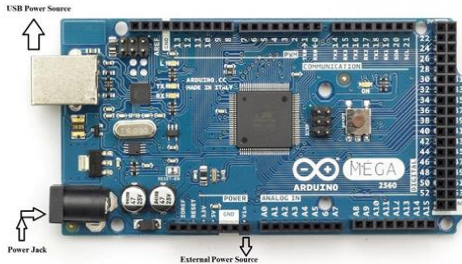
Figure-11: Power up options of Arduino mega 2560
